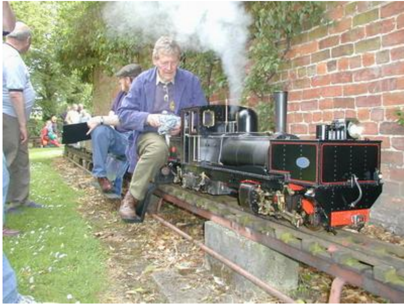
3. John Hartup and his superb 3½" gauge K1 articulated locomotive managed to achieve 4th place despite several derailments due to instability of the 30-odd truck train on curves, the heaviest load of the day. The full sized K1 was the first articulated locomotive in the world, built by Beyer Garrett of Manchester for the Tasmanian State Tramways. It is now in possession of the Welsh Highland Railway where it is being restored to full operating condition.
